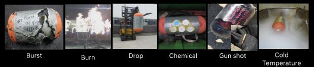
\* The hydrogen tank is completed through a number of verification tests
